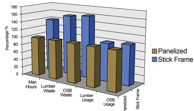
Figure 1. Relative comparison between panelized and stick framing technologies
