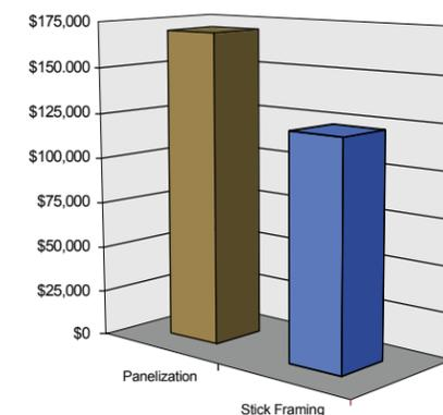
Figure 2. Estimated annual profit of five-man framing crew using different construction methods
